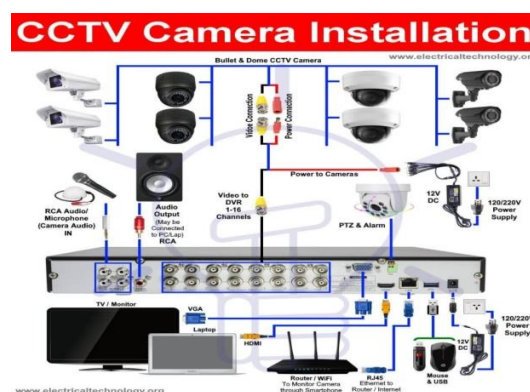
Fig: 13.9 Typical CCTV cameras security system with DVR
