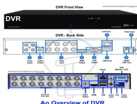
Fig :13.7 The different slots for connection on the both side of a typical DVR.
